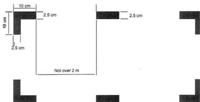
(2) If the corner markings are more than 2 m apart, intermediate lines 9 cm x 3 cm shall be inserted so that there is no more than 2 m between adjacent markings.
